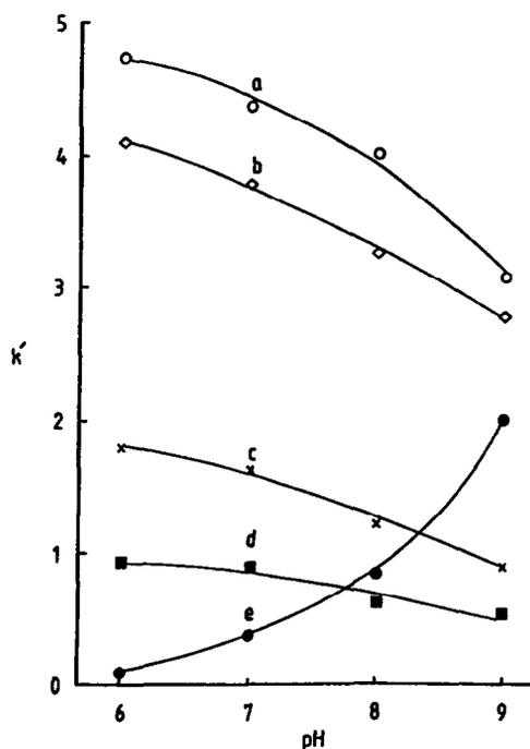
Fig. 1. Dependence of capacity factors ( $k'$ ) on pH for metal-ASPCHA chelates using TBAP-based mobile phases: (a) Mo(IV), (b) Cu(II), (c) Al(III), (d) Co(II) and (e) Fe(III).
