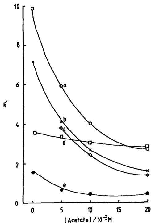
Fig. 2. Dependence of capacity factor ( $k'$ ) on acetate buffer concentration using TBAI-based mobile phase (pH 7.0): (a) Mo(VI), (b) Cu(II), (c) Ni(II), (d) Al(III) and (e) Co(II).
