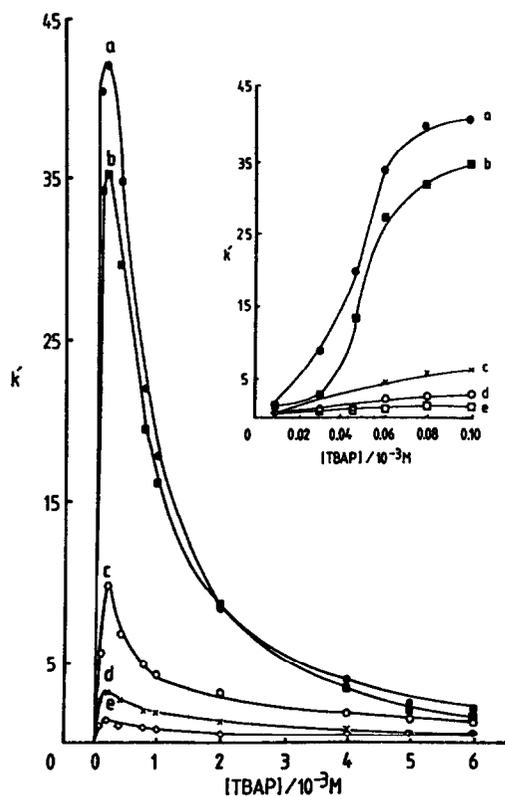
Fig. 4. Dependence of capacity factor ( $k'$ ) on pairing-ion concentration (TBAP): (a) Mo(VI), (b) Cu(II), (c) Al(III), (d) Co(II) and (e) Fe(III).
