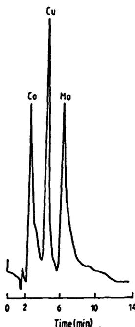
Fig. 3. Chromatographic separation of Co(II), Cu(II) and Mo(VI) as ASPHA chelates: eluent 2%  $\text{CH}_3\text{CN}$ ,  $5 \cdot 10^{-3} \text{ M}$  ASPHA,  $5 \cdot 10^{-3} \text{ M}$  TBAI,  $2 \cdot 10^{-2} \text{ M}$  acetate buffer pH 7.0; flow-rate 1 ml/min,  $20 \mu\text{l}$   $2.0 \cdot 10^{-4} \text{ M}$  Co(II), Cu(II) and  $6.0 \cdot 10^{-4} \text{ M}$  Mo(VI).
