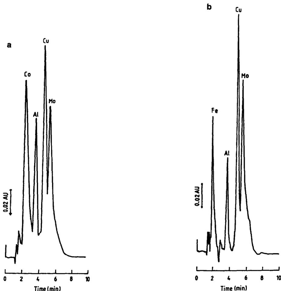
Fig. 5. Chromatographic separations of (a) Co(II), Al(III), Cu(II) and Mo(VI) and (b) Fe(III), Al(III), Cu(II) and Mo(IV) as ASPHA chelates: eluent 2%  $\text{CH}_3\text{CN}$ ,  $5 \cdot 10^{-3} M$  ASPHA,  $5 \cdot 10^{-3} M$  TBAP,  $1 \cdot 10^{-3} M$  acetate buffer pH 7.0; flow-rate 1 ml/min,  $20 \mu\text{l}$   $1.6 \cdot 10^{-4} M$  Co(II),  $4.6 \cdot 10^{-5} M$  Fe(III),  $1.5 \cdot 10^{-3} M$  Al(III),  $8.0 \cdot 10^{-5} M$  Cu(II) and  $1.6 \cdot 10^{-4} M$  Mo(VI).
